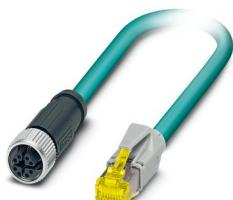
Network cable, Ethernet CAT6<sub>A</sub> (10 Gbps) CAT6<sub>A</sub> (10 Gbps), 8-position halogen-free, shielded (Advanced Shielding Technology), Plug straight RJ45 / IP20, on Socket straight M12, coding: X / IP67, cable length: 5 m
